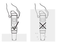
If your tester installed a spear tip electrode or flat surface electrode (refer to the *Optional Accessories* > *pH Electrodes* section) and the samples are soft solid or semi-solid, wet the sample with clean water, then slight pressure the electrode to take measure. Note that the pH-sensitive membrane must be fully touched with sample surface.
